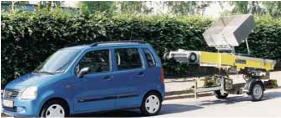
The Junior Construction Lift is suitable for transportation by nearly all types of ordinary motor vehicles
